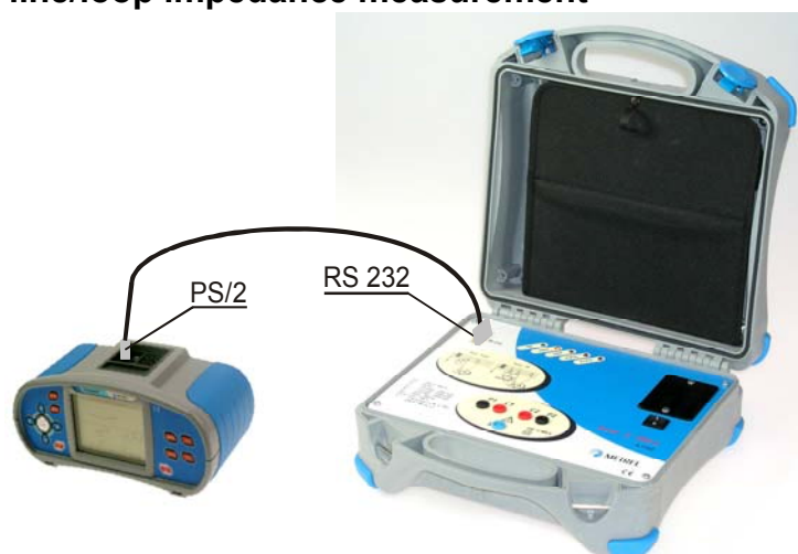
Figure 5.52: Connection of impedance adapter to the instrument
